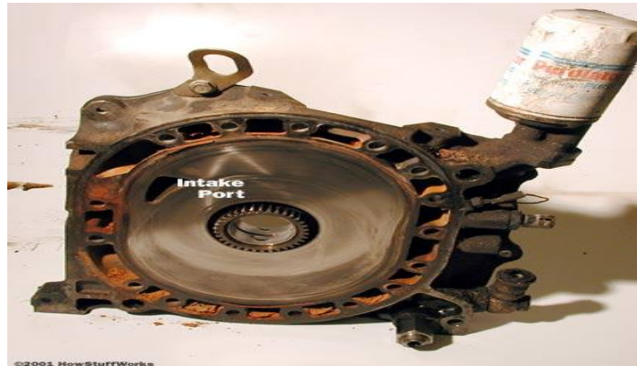
Fig 5. One of the two end pieces of a two-rotor Wankel engine
